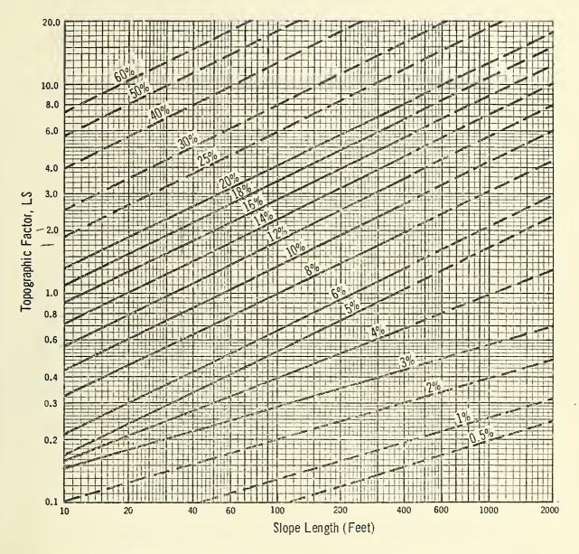
Figure 2 SLOPE-EFFECT CHART (Topographic Factor, LS)\*
